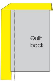
When you fold the second edge to the back the bulk of it will even out the corner and you will have a very neat mitred corner. Slipstitch the binding in place.
